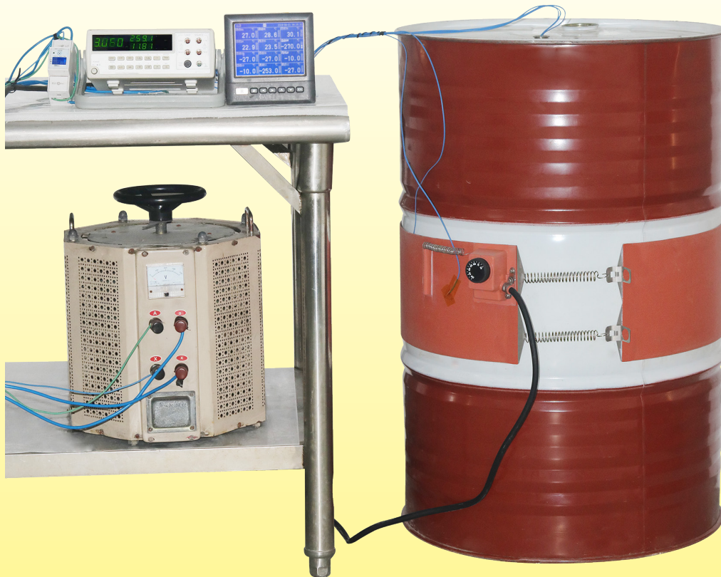
Variation in the temperature versus time of a 220-liter metal drum, filled with water, heated by a silicone heating belt 200mm wide, without thermal insulation, power 2250W (surface load 0.75W/cm 2 ).
